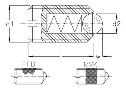
$\begin{array}{ll} d1 & = M20 \\ d2 & = 12.0 \\ Length I & = 30 \\ Spring pressure N bottom = 111.0 \\ Spring pressure N top & = 56 \\ W & = 4.5 \end{array}$
